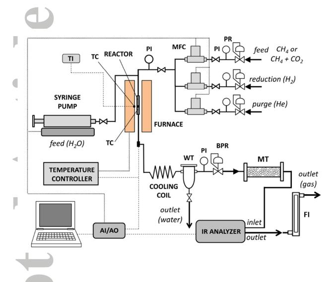
Figure 2. Experimental flow system: AI/AO – analog input/output module (analog-to-digital/digital-to-analog converter), BPR – backpressure regulator, FI – flow indicator (soap film flowmeter), IR – infrared, MFC – mass flow controller, MT – moisture trap (silica gel), PI – pressure indicator, PR – pressure reducer, TC – thermocouple, TI – temperature indicator, WT – water trap.
