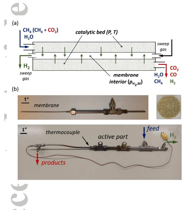
Figure 1. Membrane reactor concept (a) and the lab-scale experimental unit (b). The membrane tube (upper-left panel in Fig. 2b) dimensions were 6'' L  $\times$  1/8" OD  $\times$  0.003" W. The catalyst  $^{4}$  pellet size was 350  $\mu m$ .
