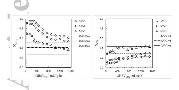
Figure 5. Effect of the feed steam-to-carbon ratio on  $CH_4$  conversion (left panel) and selectivity to CO (right panel). Equilibrium is shown by solid, dashed, and dotted lines. Operating parameters: S/C = 1-3, T = 650 °C,  $P_R = 8$  bar,  $P_M = 1$  bar,  $Q_{SG} = 200$  ml/min. All measurements were recorded after 100 h on stream.
