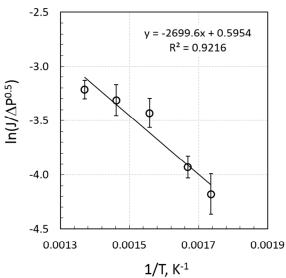
Figure 3. Membrane permeability test. The measured membrane flux is shown as a function of the pressure square root difference for various temperatures (left panel). A logarithmic plot of Eq. (5) used to estimate the activation energy and permeability coefficient is shown in the right panel.
