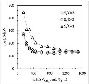
Figure 7. Membrane reactor power density (left panel) and the corresponding normalized reactor cost (right panel) as a function of space velocity for different feed steam-to-carbon ratios. Operating parameters: S/C = 1-3, T = 650 °C,  $P_R = 8$  bar,  $P_M = 1$  bar,  $Q_{SG} = 200$  ml/min. All measurements were recorded after 100 h on stream.
